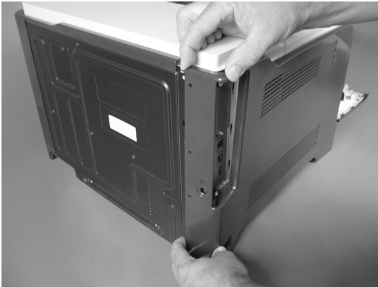
Figure 6-56 Remove the left cover (2 of 5)
