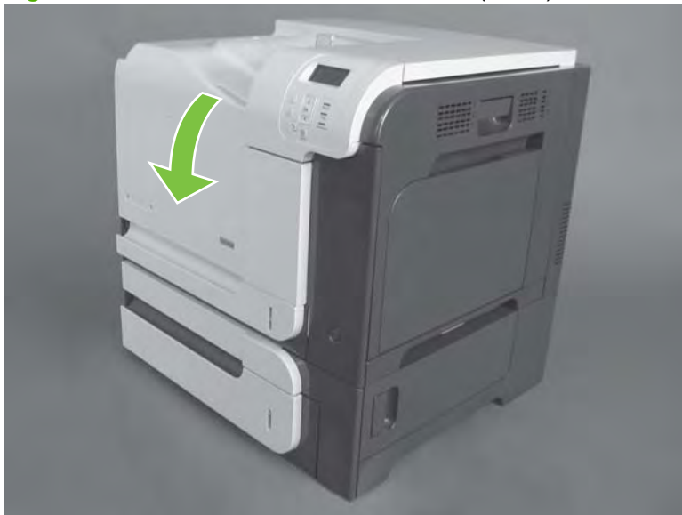
Figure 6-9 Remove the toner-collection unit (1 of 4)
