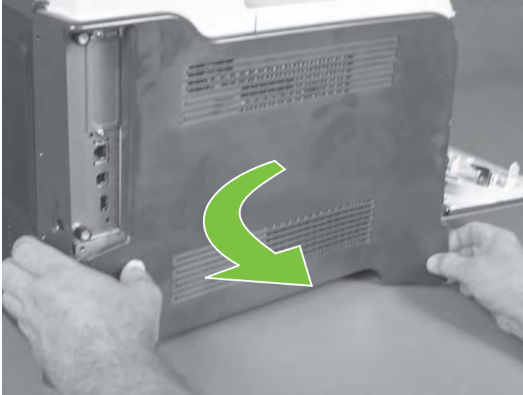
Figure 6-59 Remove the left cover (5 of 5)
