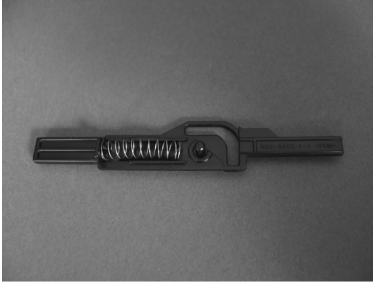
Figure 6-180 Reinstall the PGC actuators (2 of 5)
