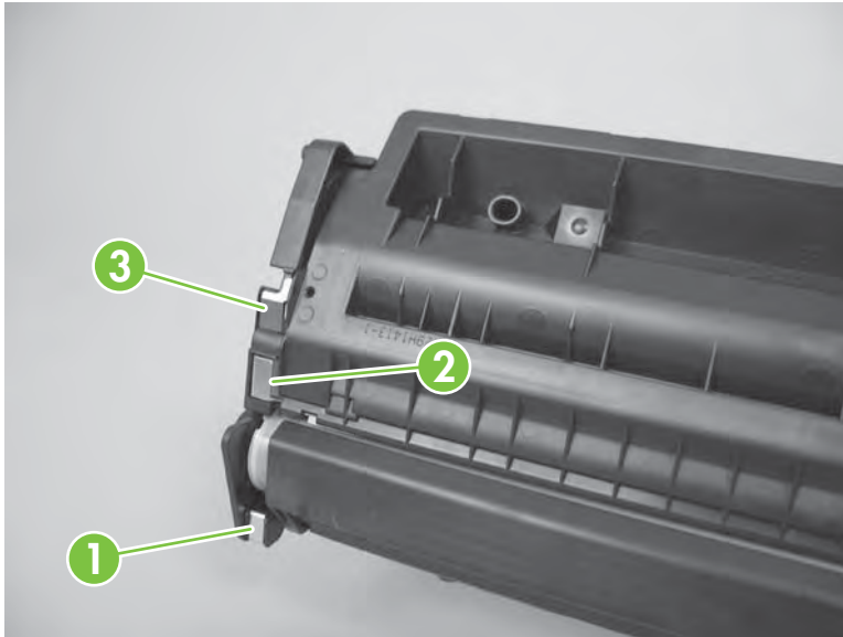
Figure 7-1 High-voltage contact points (on the print cartridge)
