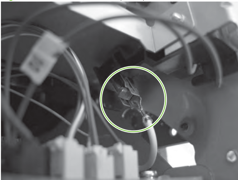
Figure 6-96 Reinstall the fuser (2 of 2)
