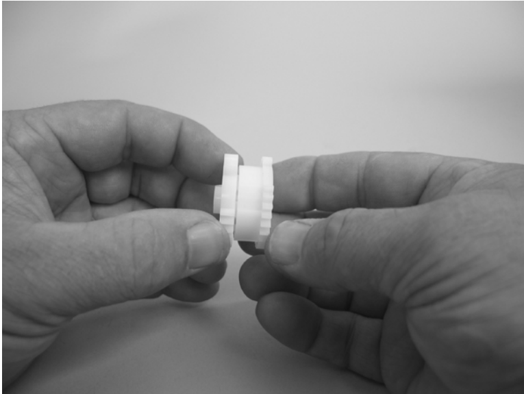
Figure 6-58 Reinstall the paper-pickup-gear assembly (3 of 3)
