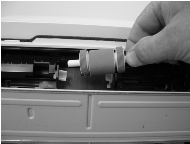
Figure 6-13 Remove the pickup roller; Tray 2 (5 of 5)
