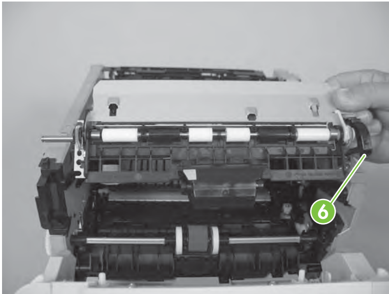
Figure 6-85 Remove the registration assembly (7 of 7)
