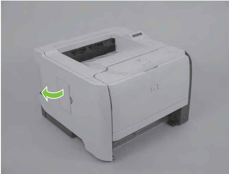
Figure 6-21 Remove the DIMM door (1 of 2; HP LaserJet P2050 Series only)
