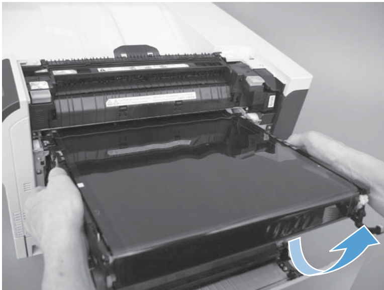
Figure 2-20 Remove the intermediate transfer belt (3 of 3)
