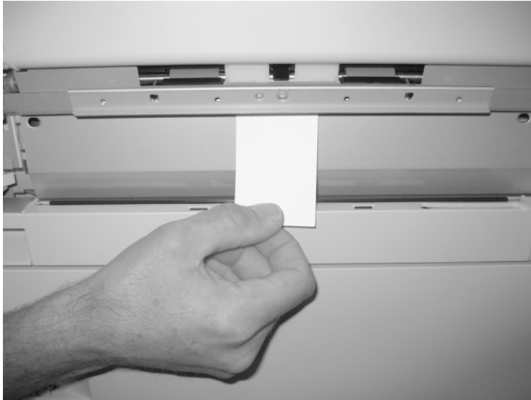
Figure 3-21 Test the Tray 3 feed sensor
