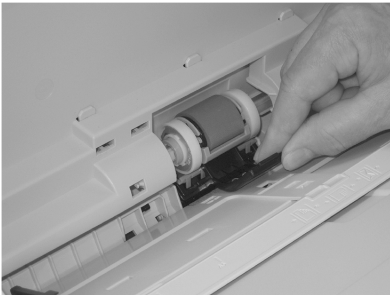
Figure 2-11 Remove the separation pad (Tray 1) (4 of 4)
