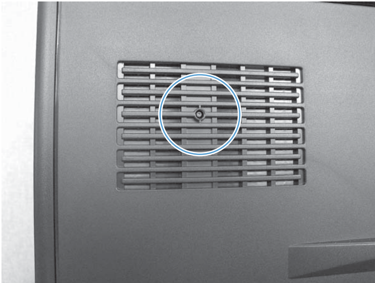
Figure 3-3 Engine test button location
