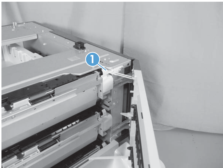
Figure 2-201 Remove the 3 x 500 right-door assembly (1 of 3)
