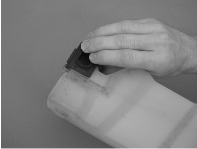
Figure 2-4 Remove the toner-collection unit (3 of 3)
