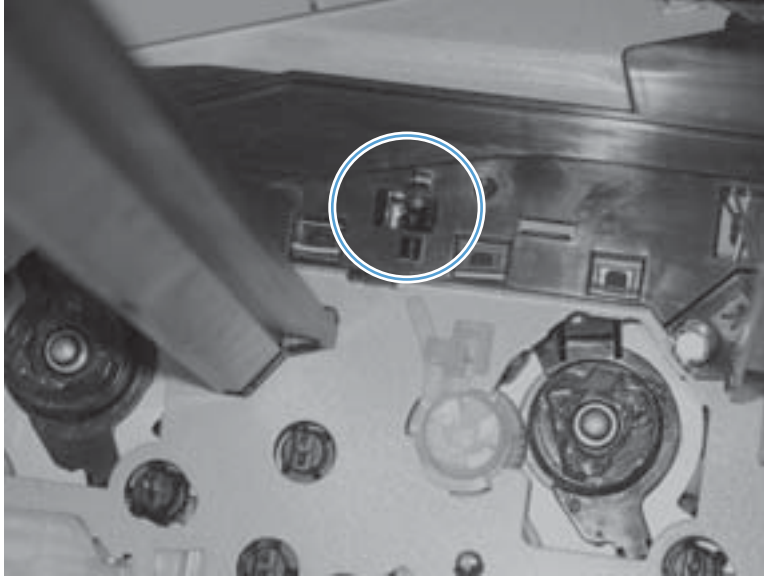
Figure 3-13 Test the ITB alienation switch
