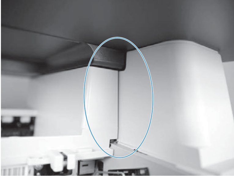
Figure 1-97 Reinstall the right cover assembly: incorrect alignment
