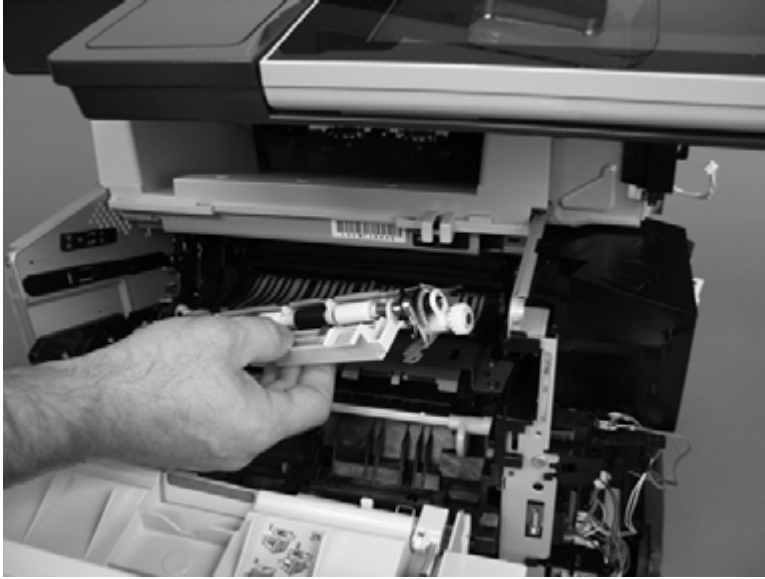
Figure 1-169 Removing the registration roller assembly (3 of 3)
