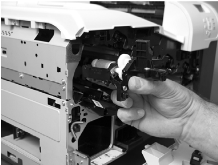
Figure 1-183 Remove the residual-toner-feed motor (7 of 7)
