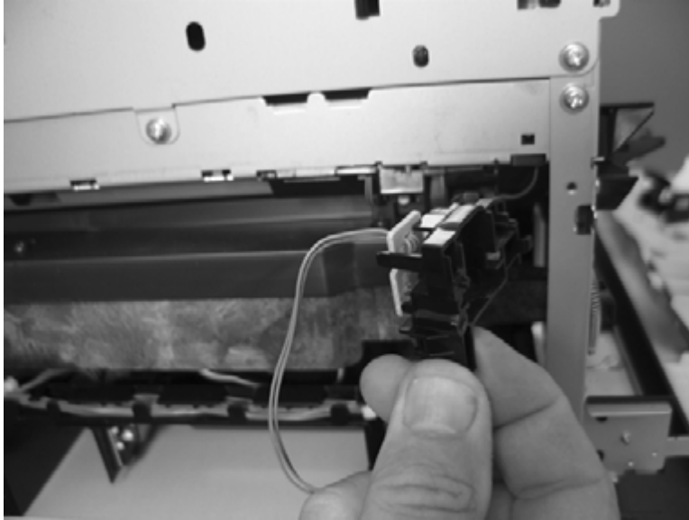
Figure 1-176 Remove the toner-collection sensor (4 of 4)
