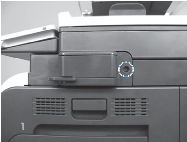
Figure 1-72 Remove the stapler cover
