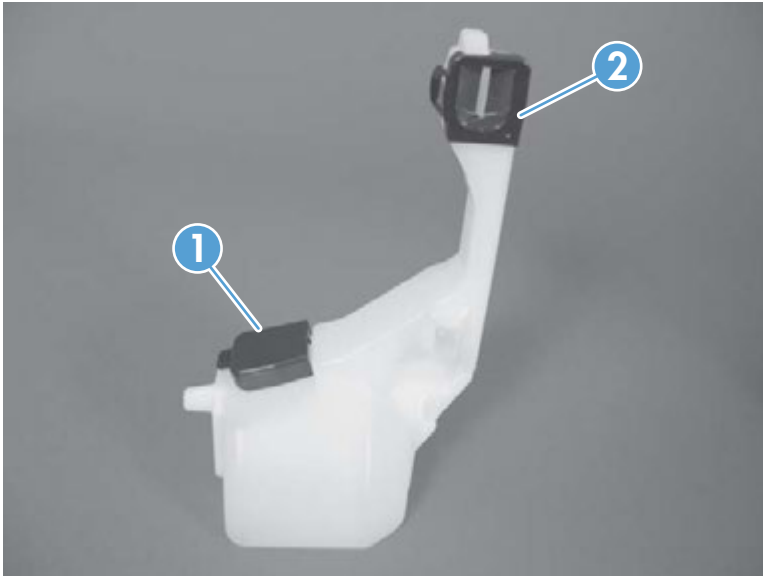
Figure 1-14 Remove the toner-collection unit (4 of 4)
