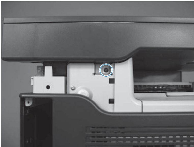
Figure 1-145 Remove the scanner assembly (3 of 6)
