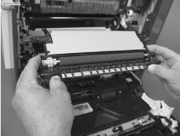
Figure 1-187 Remove the secondary transfer assembly (3 of 3)
