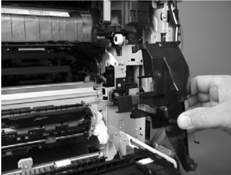
Figure 1-204 Remove the registration assembly (2 of 8)
