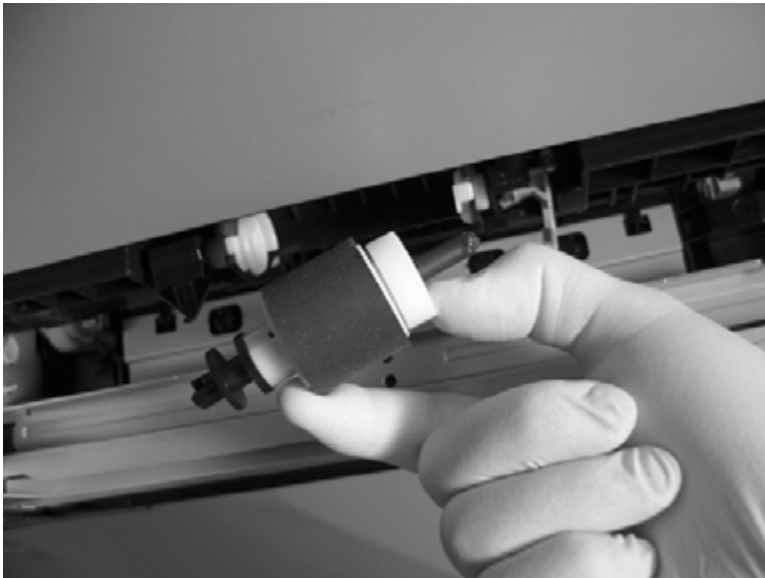
Figure 1-31 Remove the pickup roller (Tray 2) (4 of 4)
