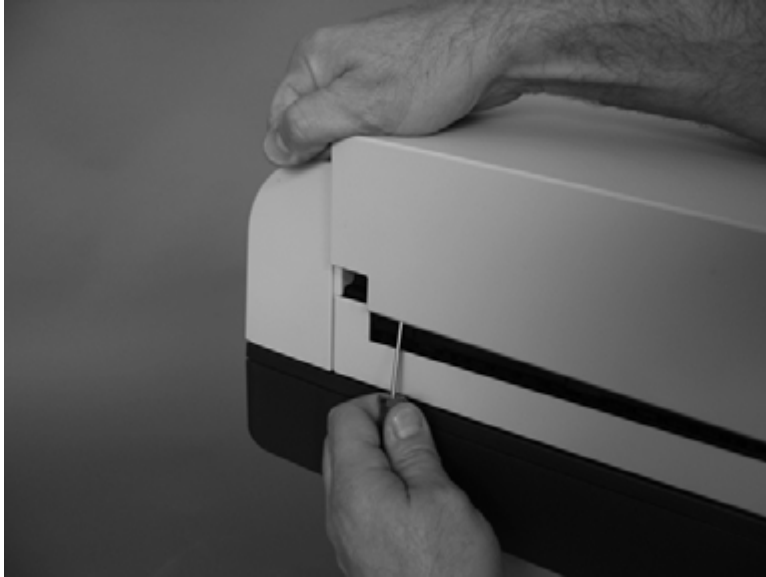
Figure 1-130 Remove the ADF jam-access cover (5 of 5)
