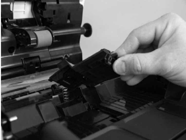
Figure 1-55 Remove the ADF separation pad and ADF separation pad spring (5 of 5)
