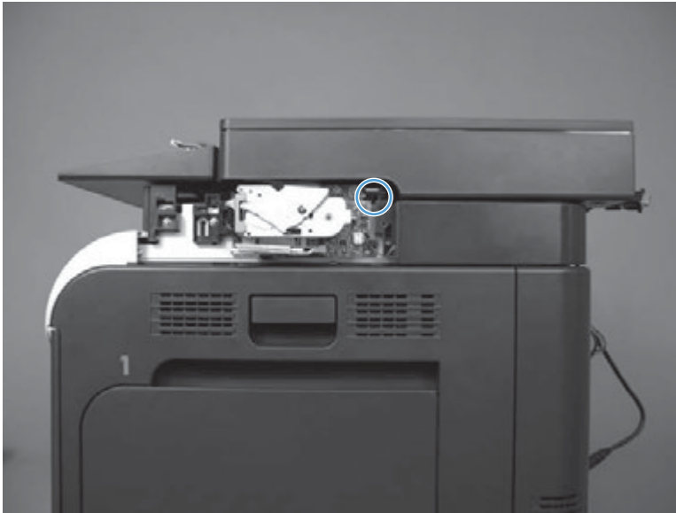
Figure 1-144 Remove the scanner assembly (2 of 6)
