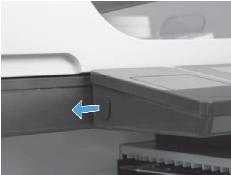
Figure 1-66 Remove USB cover
