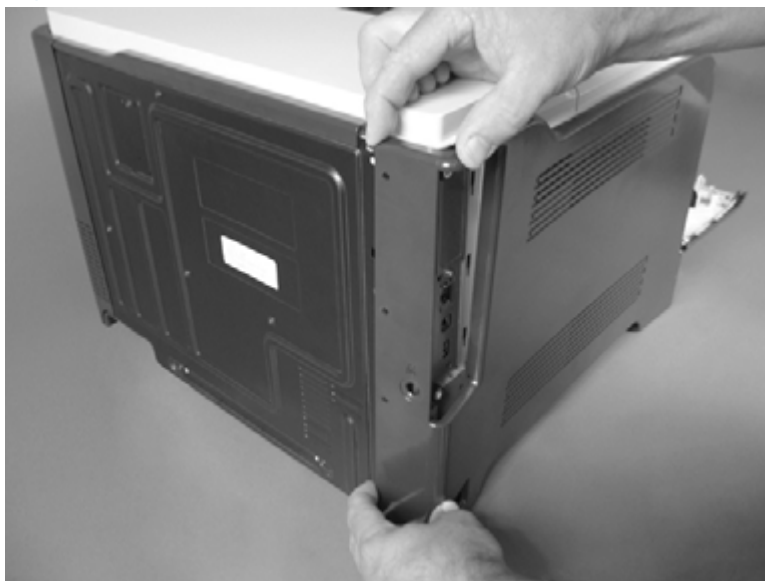
Figure 1-85 Remove the left cover (2 of 5)
