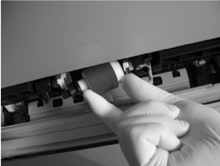
Figure 1-30 Remove the pickup roller (Tray 2) (3 of 4)
