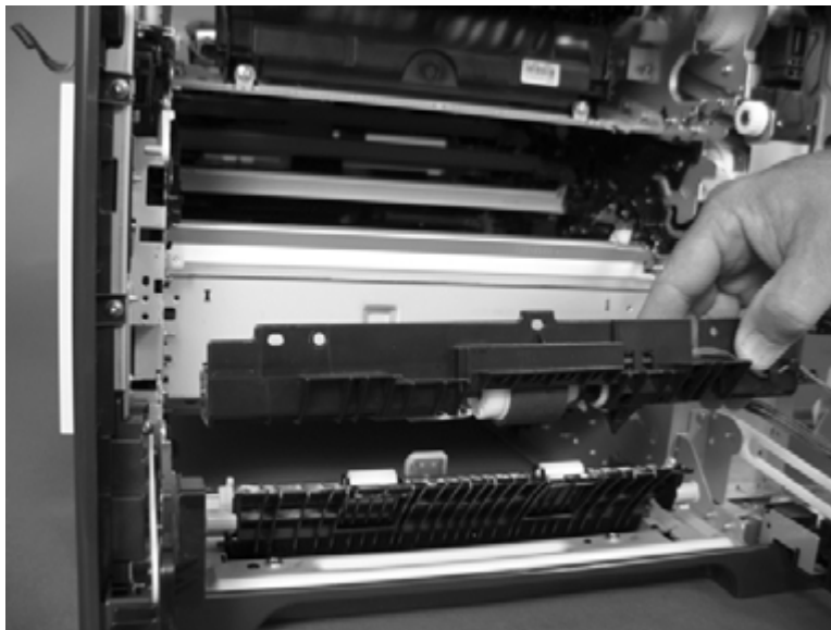
Figure 1-236 Remove the tray-pickup assembly (3 of 3)
