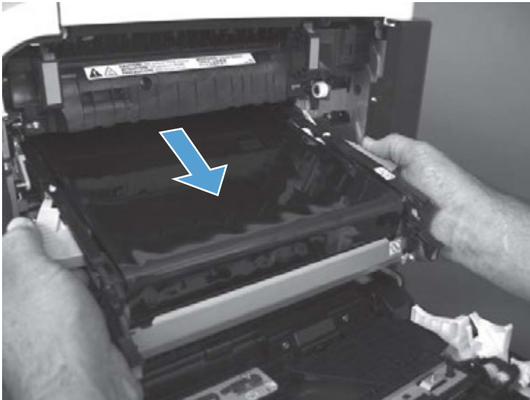
Figure 1-42 Remove the intermediate transfer belt (3 of 3)
