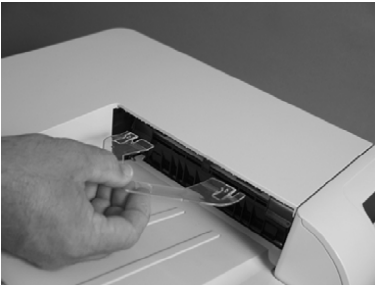
Figure 1-10 Remove the duplex-reverse guide (2 of 2)
