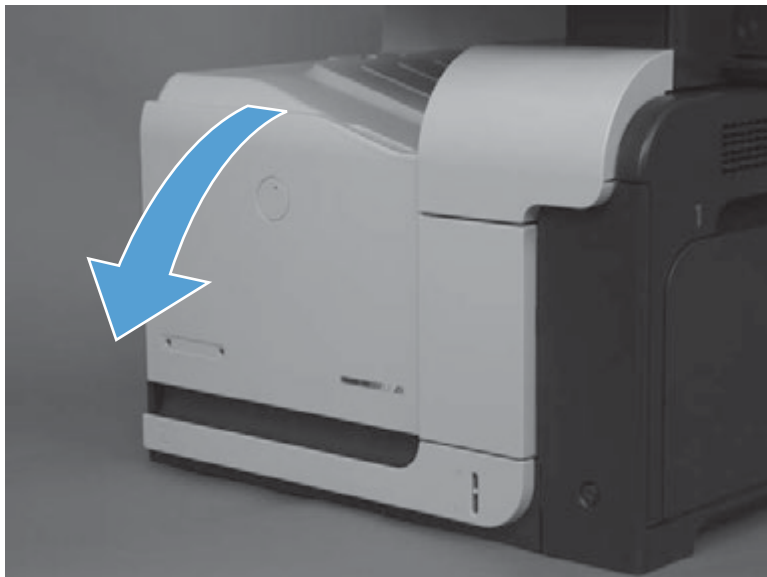
Figure 1-11 Remove the toner-collection unit (1 of 4)
