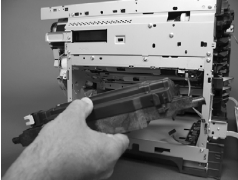
Figure 1-248 Remove the laser/scanner assembly (Y/M) (12 of 12)
