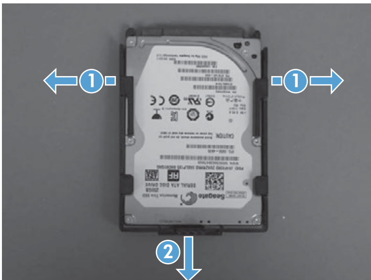
Figure 1-20 Remove the HDD (3 of 3)
