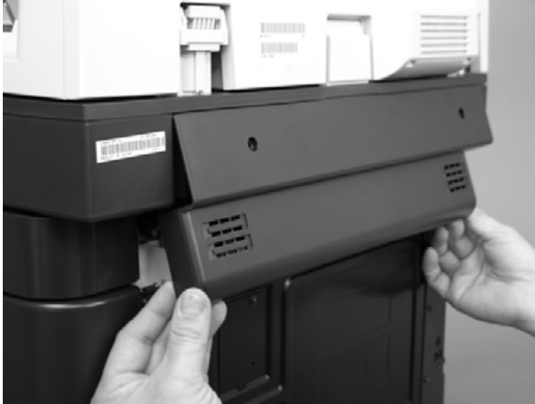
Figure 1-91 Remove the rear-upper cover (3 of 3)
