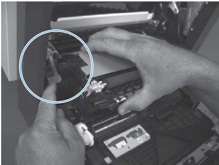
Figure 1-188 Reinstall the secondary transfer assembly
