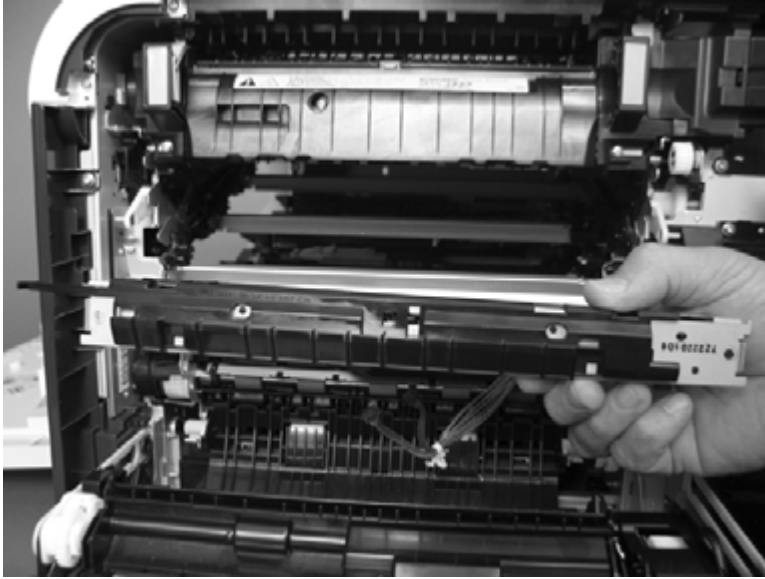
Figure 1-198 Remove the RD sensor assembly (6 of 6)
