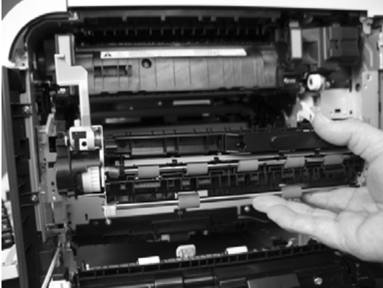
Figure 1-210 Remove the registration assembly (8 of 8)
