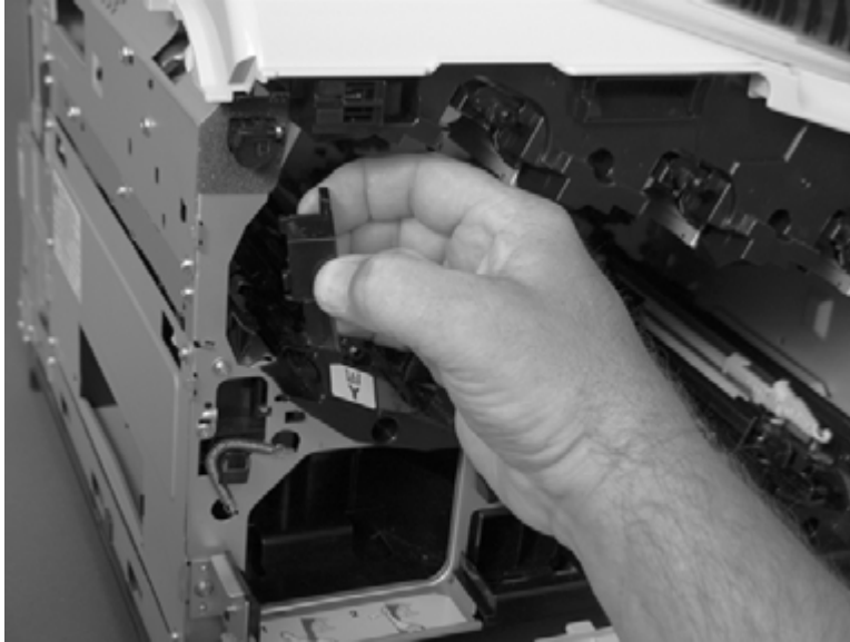
Figure 1-178 Remove the residual-toner-feed motor (2 of 7)
