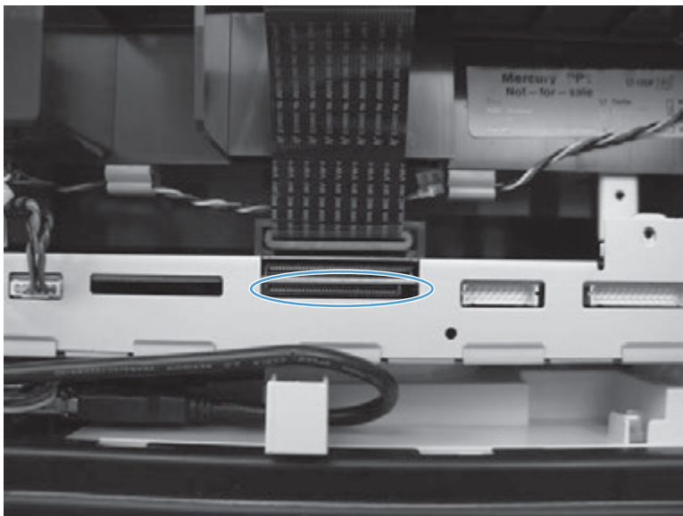
Figure 1-142 Reinstalling the SCB (2 of 2)
