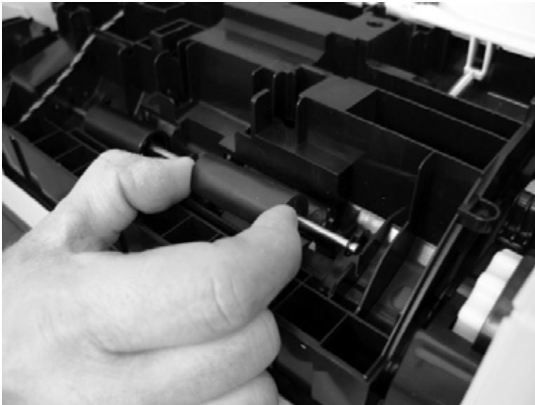
Figure 1-132 Remove the ADF roller cover (2 of 4)
