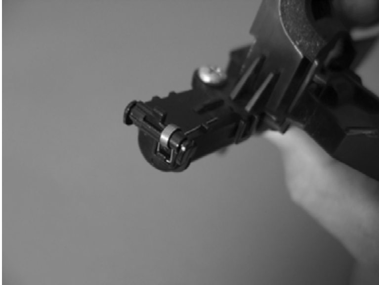
Figure 1-184 Reinstall the residual-toner collection door
