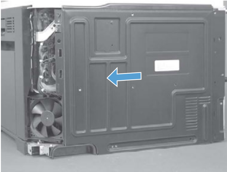
Figure 1-94 Remove the rear cover (2 of 2)
