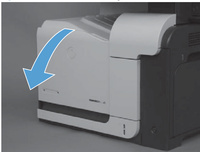
Figure 1-6 Remove the toner cartridge (1 of 2)
