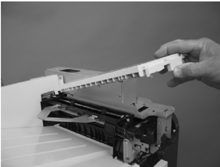
Figure 1-103 Remove the delivery cover (3 of 3)
