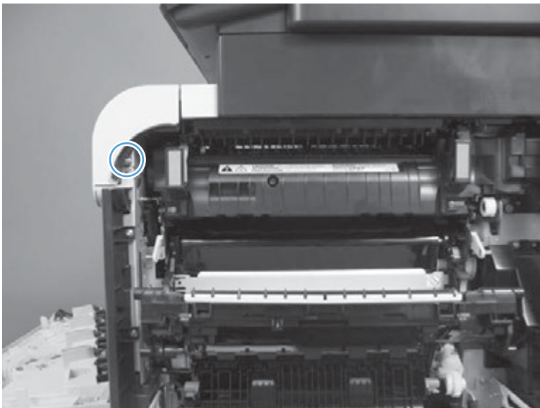
Figure 1-69 Remove the front-upper cover (2 of 4)
