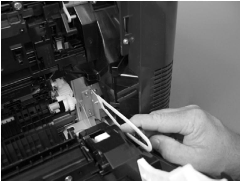
Figure 1-76 Remove the right-door assembly (4 of 8)
