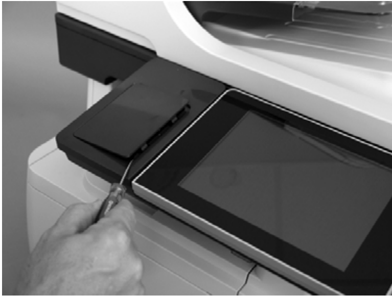
Figure 1-67 Remove the HIP cover
