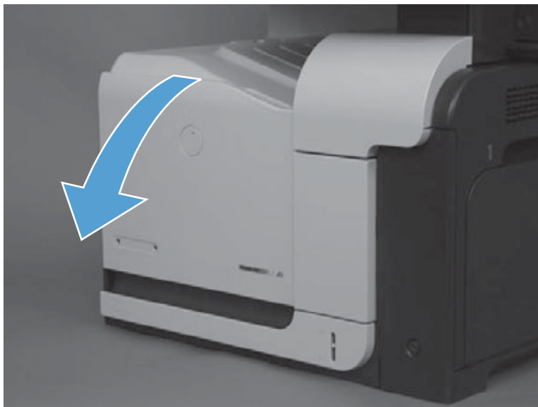
Figure 1-43 Remove the front-door assembly (1 of 2)
