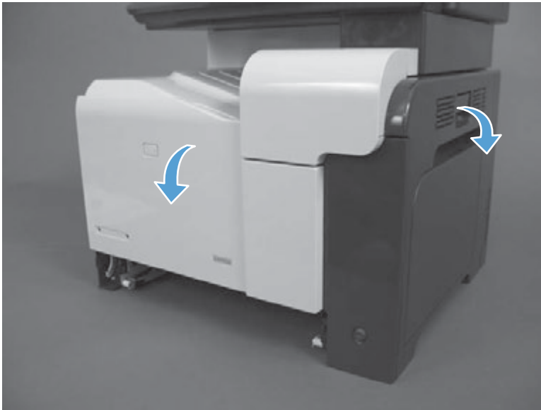
Figure 1-68 Remove the front-upper cover (1 of 4)
