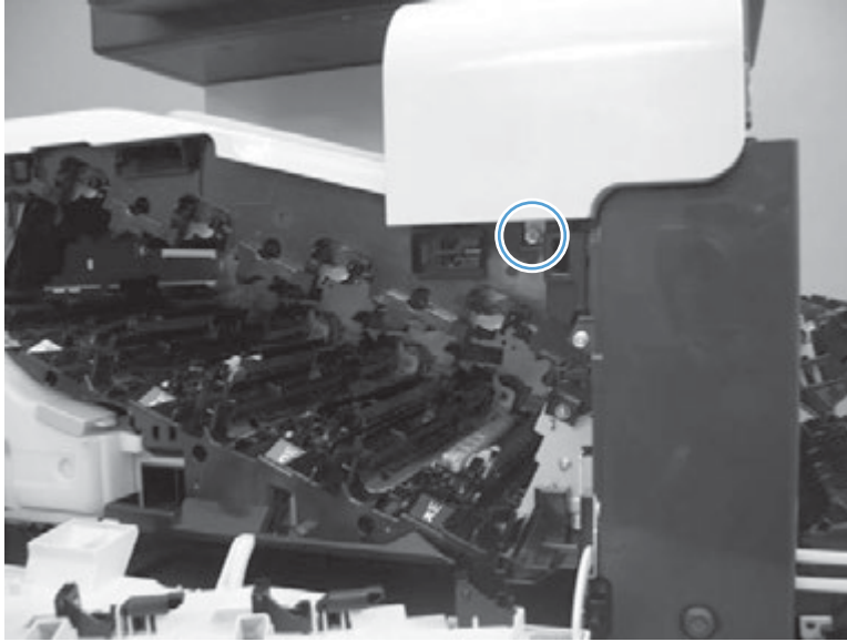
Figure 1-70 Remove the front-upper cover (3 of 4)
